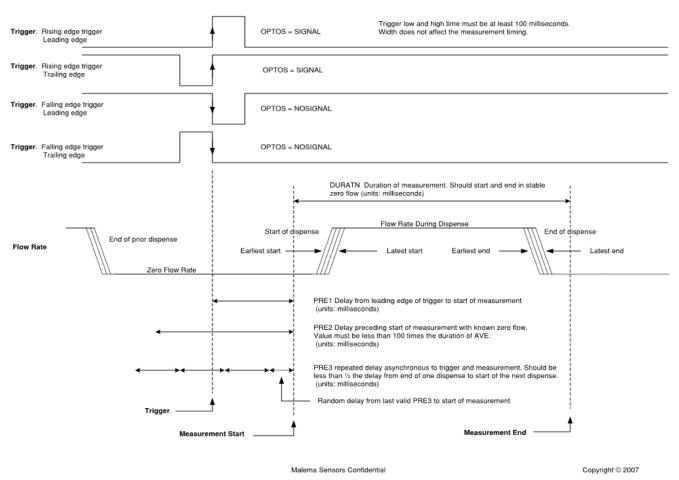
Each dispense produces a flow profile similar to the flow profile shown above. In order for the MDM-3000 to capture that flow profile and provide a precise report on the actual volume dispensed, you must describe the flow profile so the MDM-3000 knows what to look for. In order to accomplish the initial setup, you must know the following:
